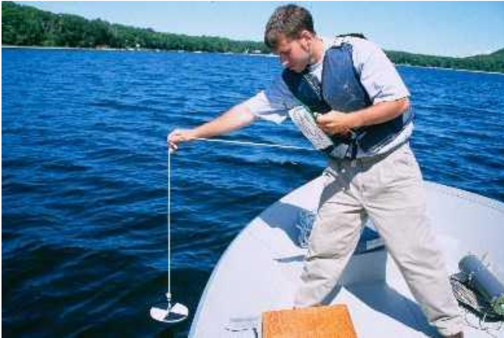
Secchi disk, unsuitable testing shallow water
