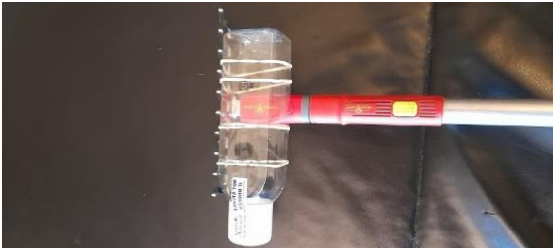
Figure 6: Secured bacterial sampling bottle on extendible (4m) Wolf Garten pole with attached rake head
