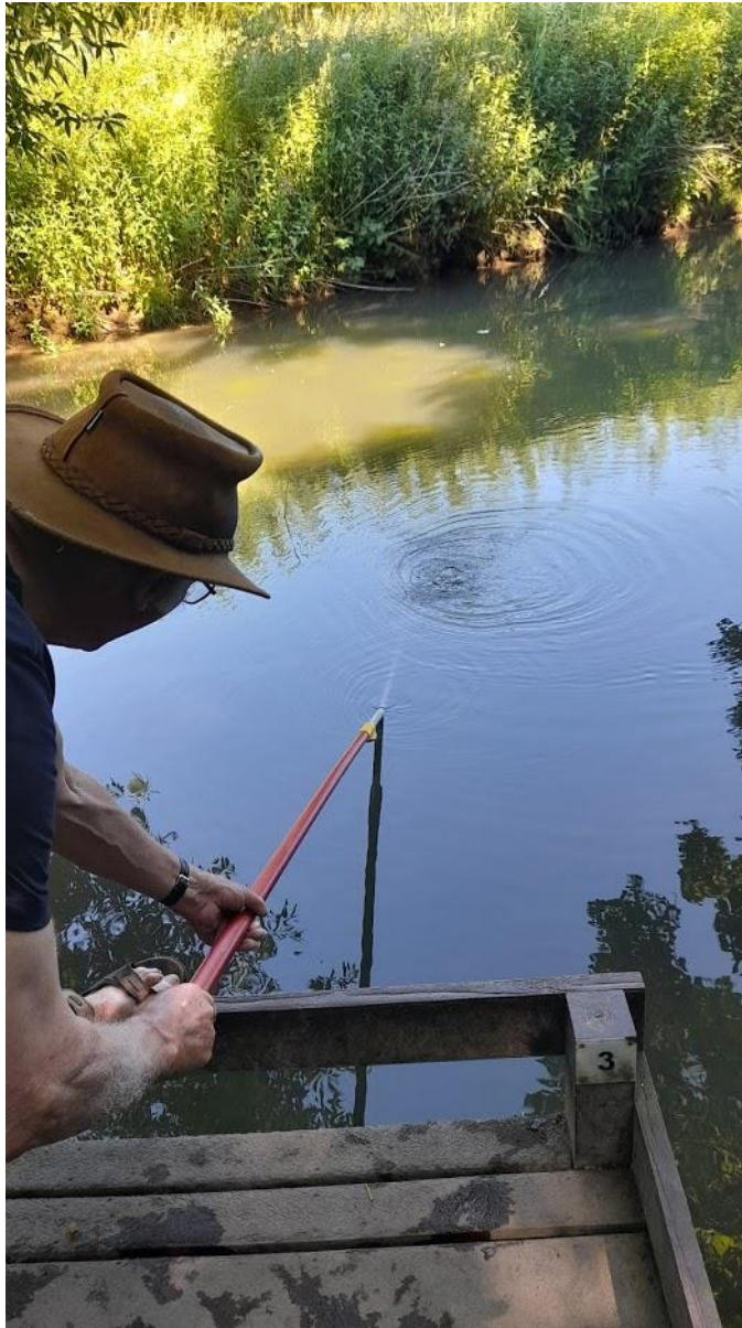
Figure 7: Below Bryon's Pool: sampling bottle immersed in river away from bank, attached to extendible pole; rate of air bubbles exiting bottle aiding judgment to adjust flow into the bottle
